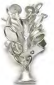
A significant factor for the economic efficiency is the low quantity of metal that must be calculated for button.
