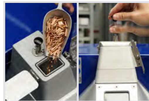
Feeding system for re-charging with constant vacuum in the melting chamber
